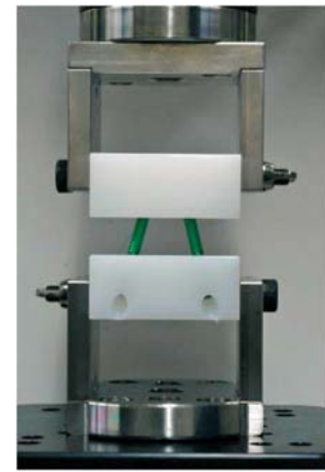
(Figure 3) ASTM F1717-04 for GO-LIF
