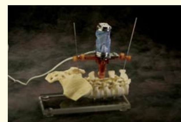
Figure 3: The SpineAssist Device mounted on a model of the lumbar spine with the spinous process clamp and multi-level bridge
